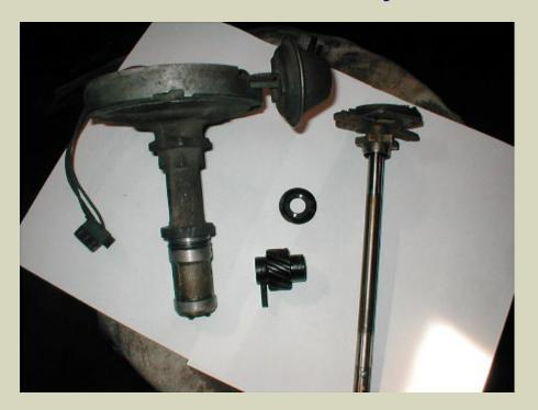
The underside of the shaft has 6 evenly spaced "lobes" that cause the distributor to fire normally. Place the rotor on the shaft properly and find the point that faces towards the tip of the rotor assembly. Now make a "triangle" across the other points and mark the points that are NOT in the triangle. These 3 points will be carefully ground off the shaft. (Only 2 are shown in the picture below. The third is behind the shaft.)
